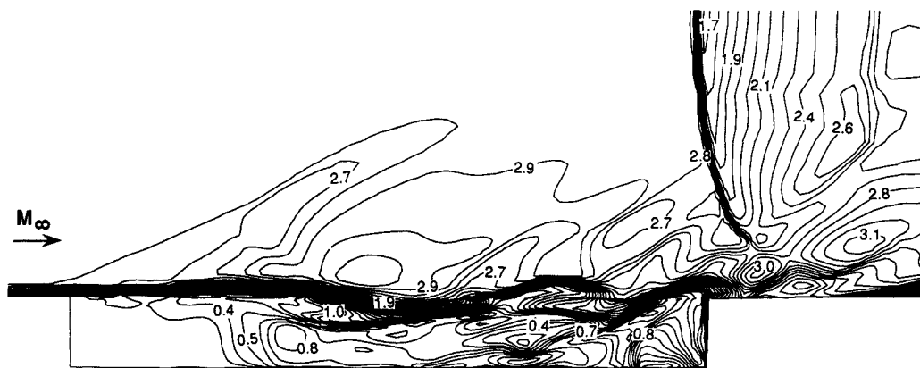
Fig. 5 Instantaneous Mach contours of the longitudinal plane located 1.0 in. from the symmetry plane for case 1.
